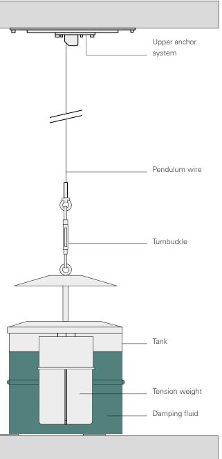
The direct hanging pendulum is a gravity-referenced instrument, composed by:
